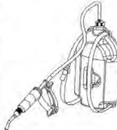
Figure 2: 5L bottle and applicator device with tubing
